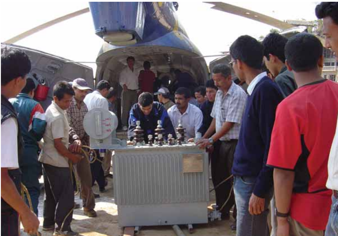
Transportation of Distribution Transformer to Remote Areas by Helicopter
